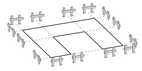
49. For the following foundation, place batter boards as needed to string every line.
