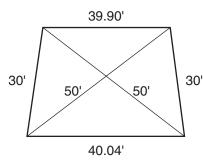
As you can see here, the two diagonals are the same length, but the corners are obviously not square with each other. This is why a surveyor cannot depend on such a method to make 90 degree corners. Using the 3/4/5 triangle method would be much more accurate.
